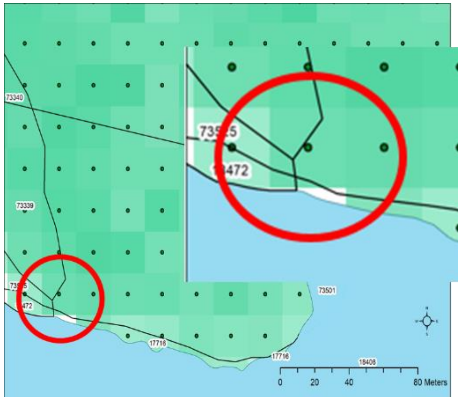
Figure 17 - Example of a raster pixel being bisected into 4 by polygon boundaries with only one polygon including the centroid value.
